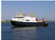
2.2.7 The 'Earls', as the above two vessels are affectionately known, are sister ships which were specifically designed to serve the Outer North Isles roster. Their most distinguishing feature is the large lifting derrick affixed to the upper superstructure. The derrick is required for the
