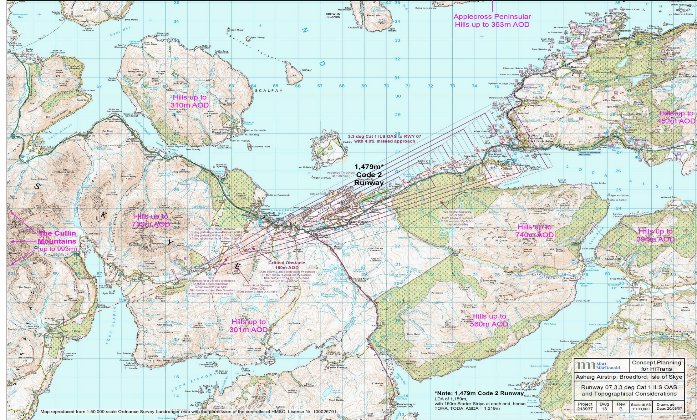
Figure 2 Standard Precision Approach Obstacle Limitation Surfaces
