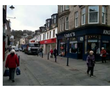
1A - Bollards indicate separation of road users which should be removed to create a shared space
