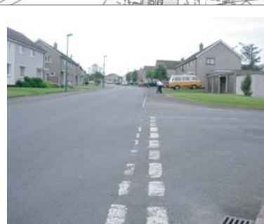
5b Junction mouths on Castlegreen Road could be reduced in width to aid pedestrians. Further investigation is needed to determine how this local distributor road can be made more cycle friendly.
