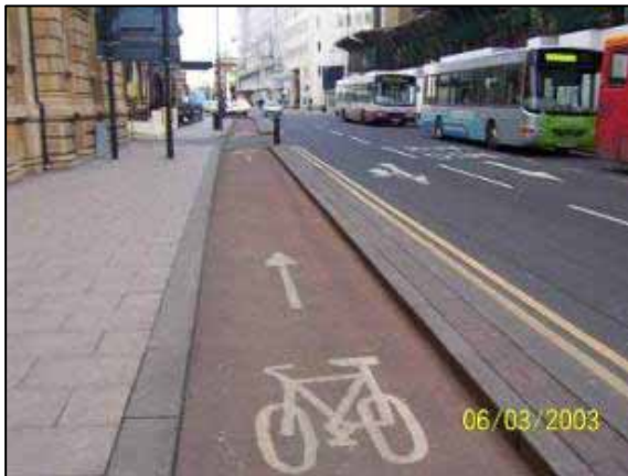
Figure 5-7: One way streets in Inverness present major barriers to cycling, the preferred solution would be segregated contra-flow cycle lanes such as Wellington Street in Leeds (photo courtesy of Cycling England).
