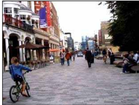
Figure 5-14: New Road in Brighton showing an example of shared space in practice (photo courtesy of Cycling England)
