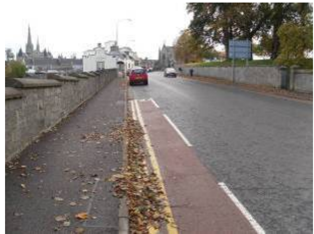
Figure 3-11: Short section of cycle lane on Bridge Street leading to High Street which ends before reaching any trip generators
