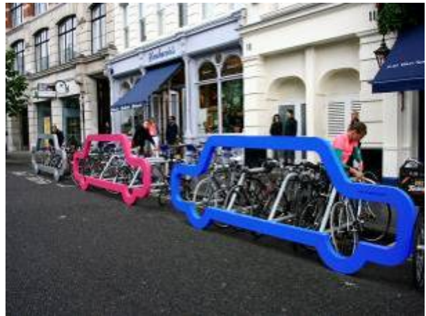
Figure 5-53: Less conventional cycle parking, shaped as a car, removing one parking space and installing one car shaped bike rack can provide parking for up to 10 bikes (Cyclehoop) 10
