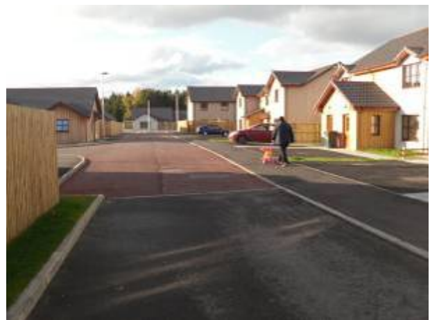
Figure 5-57: New housing in Pilmuir shows traffic calmed streets with wide shared footways
