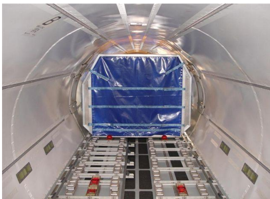
ULD and roller floors on ATP
