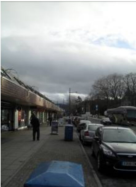
Figure 5-12: Cluttered footways reduce effective widths
