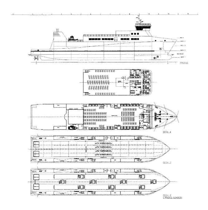
Note: power-plants are located well aft to facilitate rapid access and replacement in the event of failure or routine maintenance, thereby reducing disruption to service..
