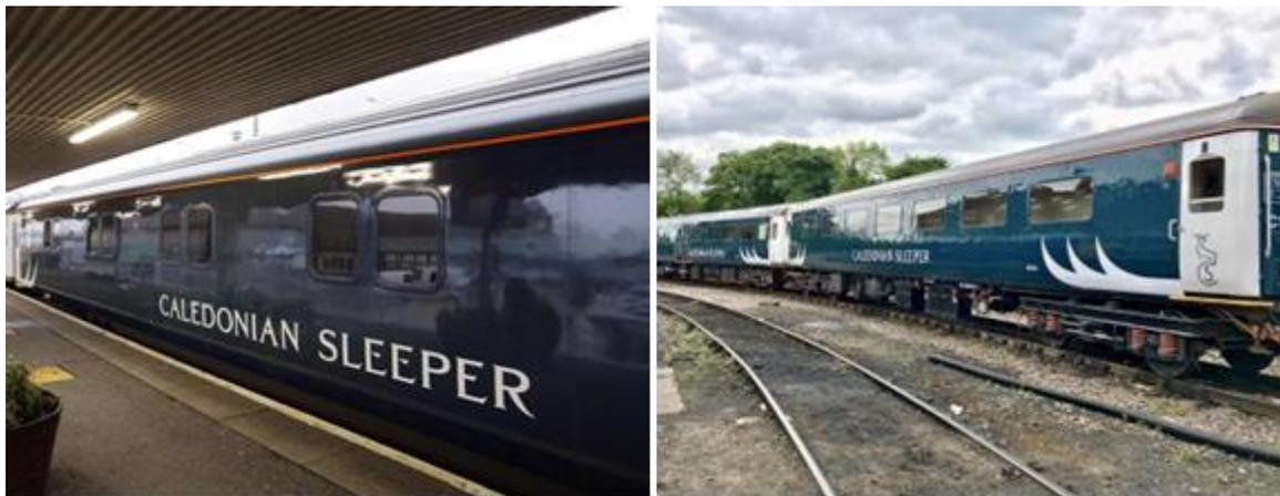
Figure 2: Vinyl Wrap Mark 3 Sleeper (Left) and Painted Mark 2 BSO (Right) [1]
