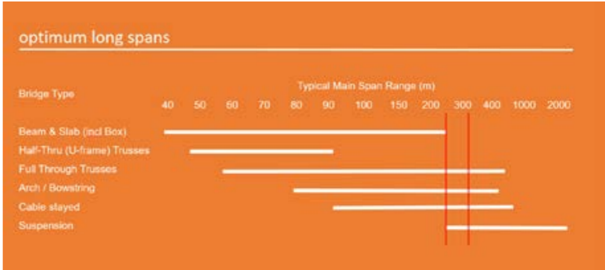
Figure 16: Bridge Spans and Structural Options
