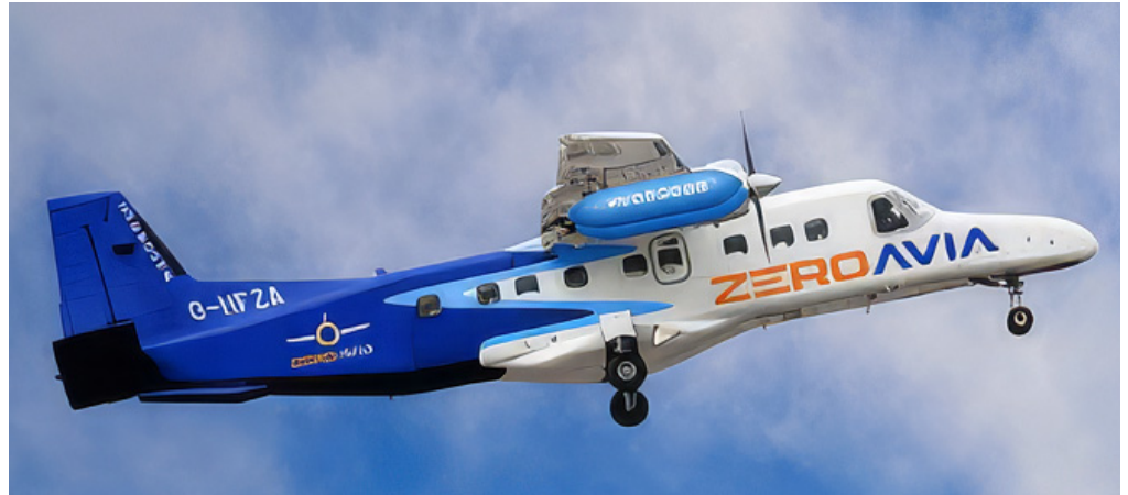
Figure 5: Example of a hydrogen aircraft produced by Zeroavia. Image credit: Zeroavia.
